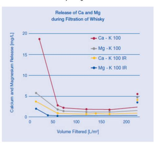
The following total calcium and magnesium release per m² filter sheet at a flow velocity of 500 L/m²/h (12.3 gal/ft2/h) was calculated during this filtration run:
